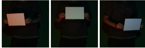
Fig. 3. Calibration sequence: from the corners of the white balance card the plane’s varying normal can be computed and used to calibrate light sources.
