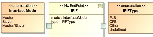
Fig. 7. Modeling of the IPIF hardware wrapper
