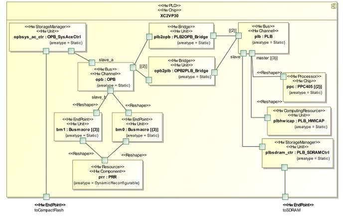
Fig. 15. Modeling of a PLB ICAP based Reconfigurable Architecture
