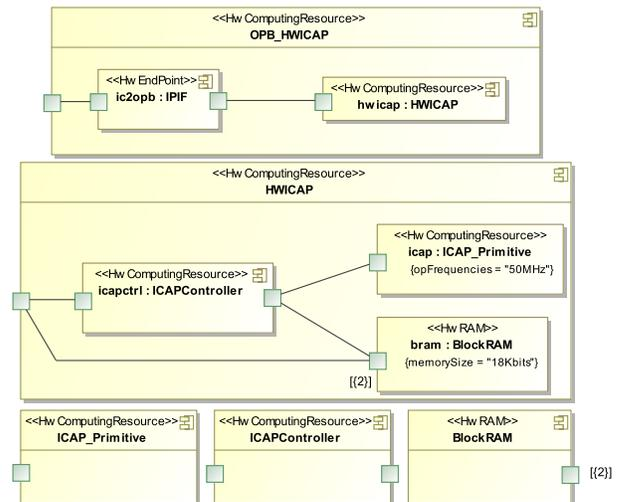
Fig. 9. Modeling of the OPB HWICAP Peripheral
