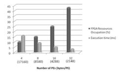
Fig. 8. System scalability/performance running a picture rotation algorithm on a Stratix 2S180
