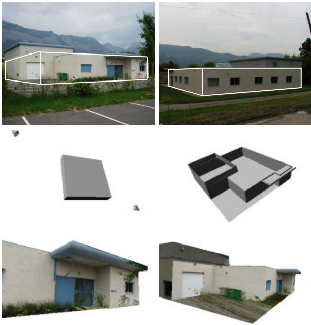
Figure 6: Opposite viewpoints scene: (top) the original images used for the reconstruction; (middle) the reconstruction scenario with the computed model and the cameras' positions; (bottom) new viewpoints of the model.
