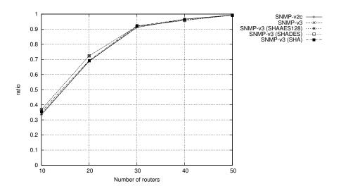
Figure 10: Delivery ratio of SNMP messages
