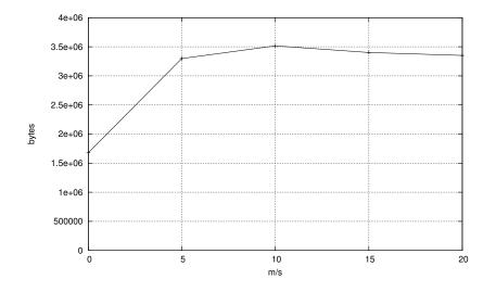
Figure 3: OLSRv2 accumulated control traffic throughout the simulation in a network with 50 routers and variable router velocity.
