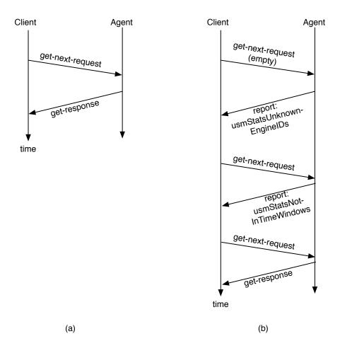
Figure 6: SNMP message exchange: (a) in SNMPv2 (b) in SNMPv3 with privacy
