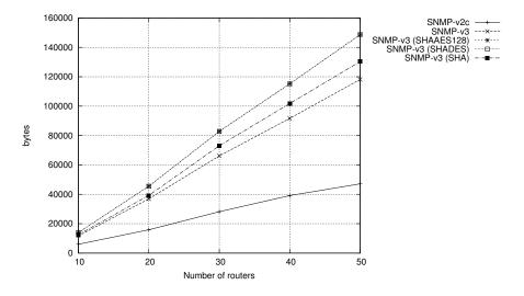
Figure 4: Accumulated SNMP traffic overhead
