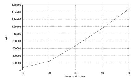
Figure 2: OLSRv2 accumulated control traffic throughout the simulation
