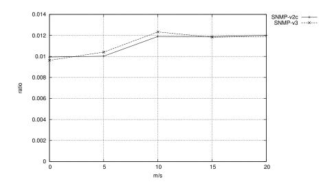
Figure 8: MAC collision ratio in a network with 50 routers and variable router velocity.
