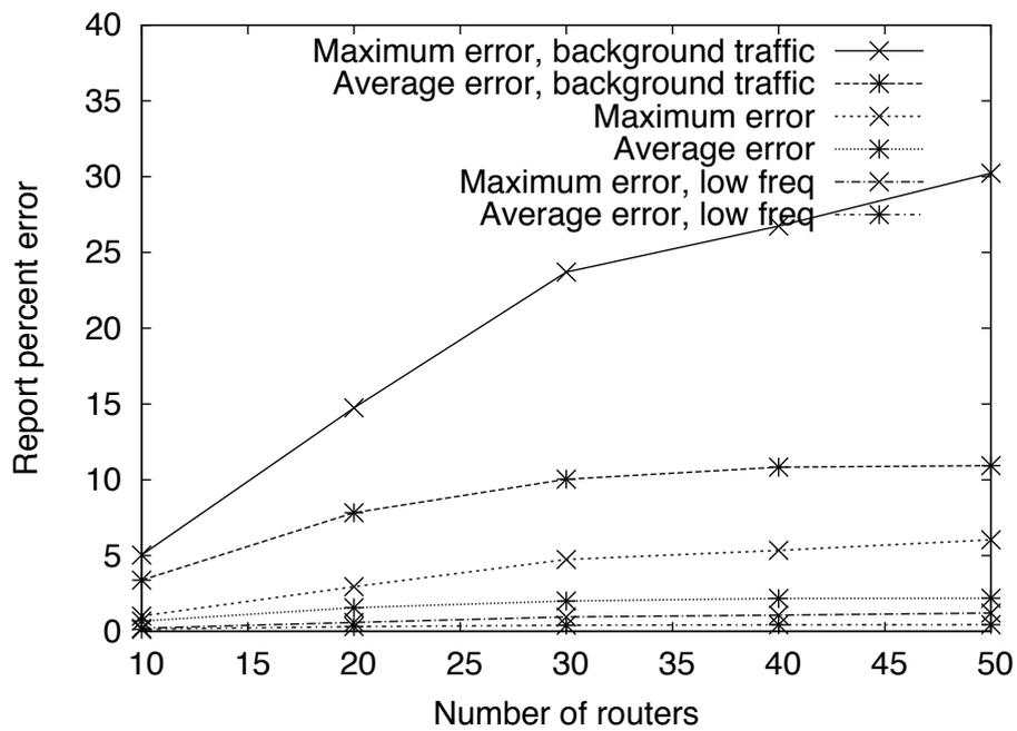
Figure 15: The typical and maximum error in standard SNMP performance reporting.
