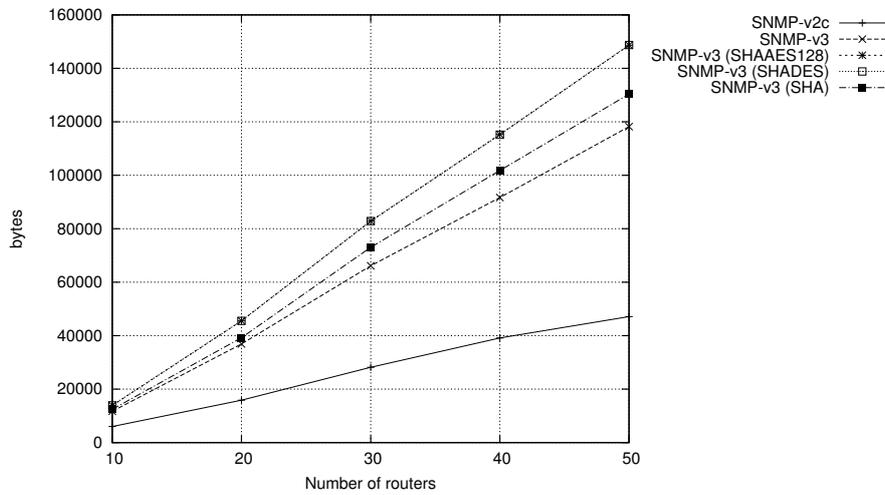
Figure 4: Accumulated SNMP traffic overhead
