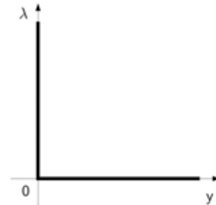
Figure 1. Complementarity condition as a constitutive law for an ideal diode
