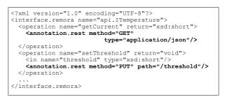
Figure 5: Mapping the REST verbs to equivalent Remora operations and identifying content types.
