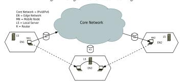
Fig. 3. Simultaneous Mobile Nodes Roaming towards same Edge Network.
