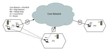
Fig. 2. Single Mobile Node Roaming.
