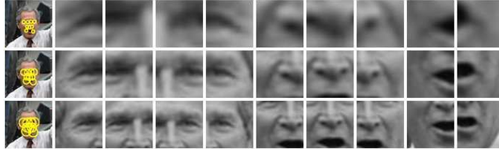
Figure 5: Illustration of our SIFT-based face descriptor. SIFT features (128D) are extracted at 9 locations and 3 scales. Each row represents a scale at which the patches are extracted: the top row is scale 1, the middle row is scale 2 and the bottom row is scale 3. The first column shows the locations of the facial features, and the remaining nine columns show the corresponding patches on which 128D SIFT descriptors are computed. The descriptor is the concatenation of these 3 \times 9 SIFT features.
