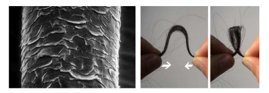
Figure 1.1: Left, close view of a hair fiber (root upwards) showing the cuticle covered by overlapping scales. Right, bending and twisting instabilities observed when compressing a small wisp.
