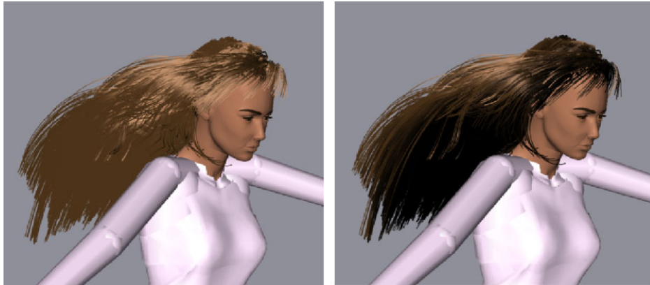
Figure 4.6: Interactive hair self-shadowing processed by accumulating transmittance values through a light-oriented voxel grid [BMC05]. (left) Animated hair without self-shadows; (right) Animated hair with self-shadows.
