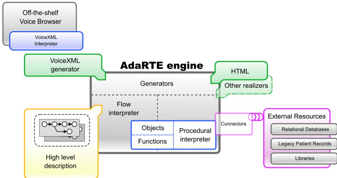
Figure 1 Block diagram of the AdaRTE architecture.
