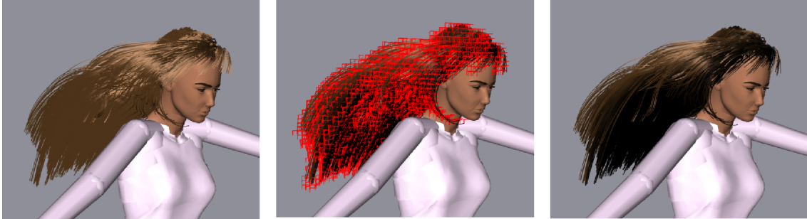
Figure 1: A dynamic hair without self-shadowing (left) and shaded with our algorithm (right). The 3D light-oriented map storing hair density and transmittance (middle). The whole simulation (including animation and our rendering) is running interactively on a standard CPU.
