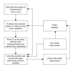
Fig. 1. The procedure for fault diagnosis
