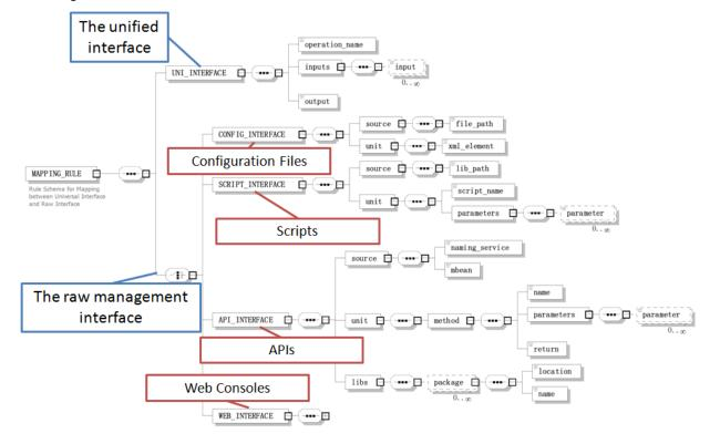
Figure 3. the Mapping Rule for Middleware Management Interfaces
