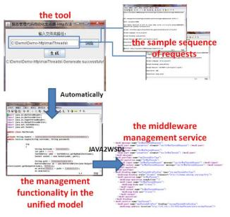
Figure 8. The Tool for Management Services Encapsulation
