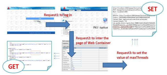
Figure 6. the Mapping Rule for Web Consoles
