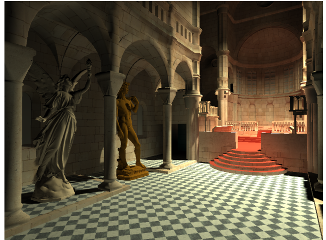
Figure 1: This global illumination visualization runs 7.2 FPS at 960 \times 720 resolution. The direct-to-indirect transport operator was precomputed in 31 minutes for the Sibenik cathedral with Lucy and David statues (1.2M triangles) using our meshless finite element method. Per-pixel direct lighting was rendered using shadow maps. The viewpoint and light source can be freely moved at runtime.
