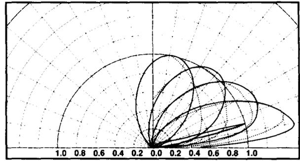
Figure 8: Normalized BRDF's of roughened aluminum as obtained from theory (solid lines) and experiment (dashed lines) for incidence angles of  $\theta_i = 10^\circ, 30^\circ, 45^\circ, 60^\circ,$  and  $75^\circ$ .  $\lambda = 0.5\mu m$ . This is the same surface as in Figure 7. The surface shows strong directional diffuse and emerging specular reflection at this wavelength.
