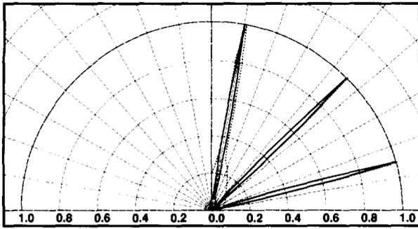
Figure 7: Normalized BRDF's of roughened aluminum as obtained from theory (solid lines) and experiment (dashed lines) for incidence angles of  $\theta_i = 10^\circ, 45^\circ,$  and  $75^\circ$ .  $\lambda = 2.0\mu m$ . This is the same surface as in Figure 8. The surface shows strong specular reflection at this wavelength.
