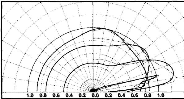
Figure 9: Normalized BRDF's of roughened magnesium oxide ceramic as obtained from theory (solid lines) and experiment (dashed lines) for incidence angles of  $\theta_i = 10^\circ, 45^\circ, 60^\circ,$  and  $75^\circ$ .  $\lambda = 0.5\mu m$ . The surface shows strong uniform diffuse and emerging specular reflection.
