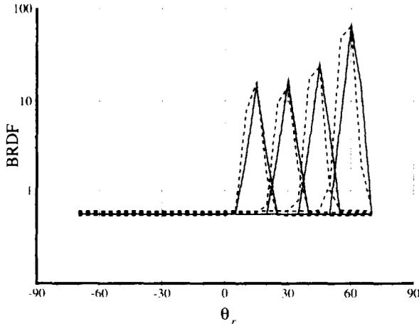
Figure 11: Absolute BRDF's for smooth blue plastic as obtained from theory (solid lines) and experiment (dashed lines) for incidence angles of  $\theta_i = 15^\circ, 30^\circ, 45^\circ,$  and  $60^\circ$ .  $\lambda = 0.46\mu\text{m}$ . This surface shows a typical smooth plastic reflection pattern with combined specular and uniform diffuse behavior.
