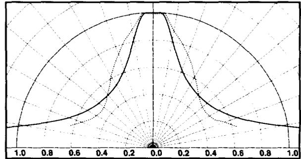
Figure 10: Normalized BRDF's of sandpaper as obtained from theory (solid lines) and experiment (dashed lines) for normal incidence,  $\theta_i = 0^\circ$ .  $\lambda = 0.5\mu m$ . The surface shows a large reflectance at grazing reflection angles.
