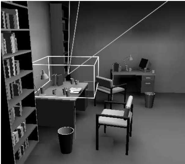
Figure 6: Example of a cluster, with links to other radiative elements.
