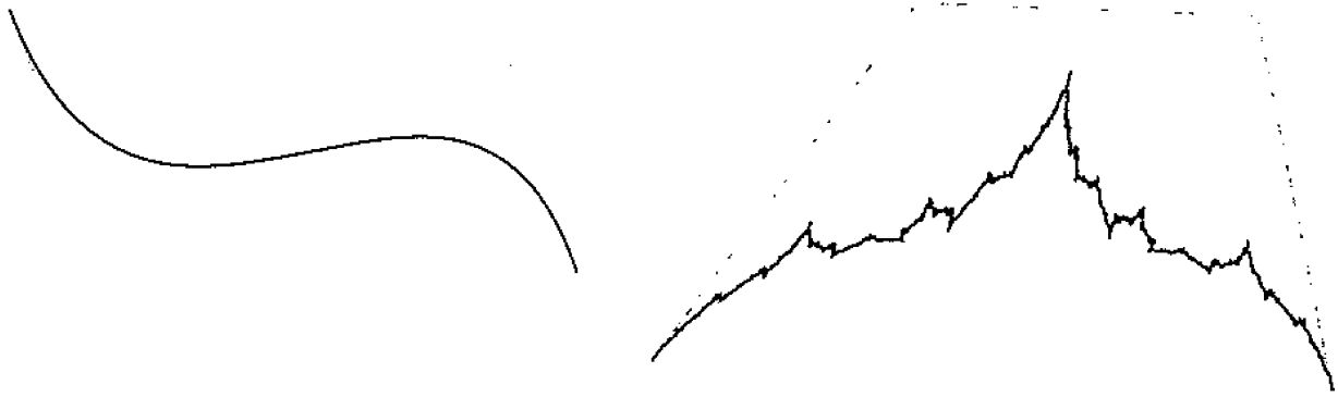
Fig. 5.1. Bézier and fractal curves obtained as IFS attractors. The fractal curve is controlled in the same way as the Bézier curve.
