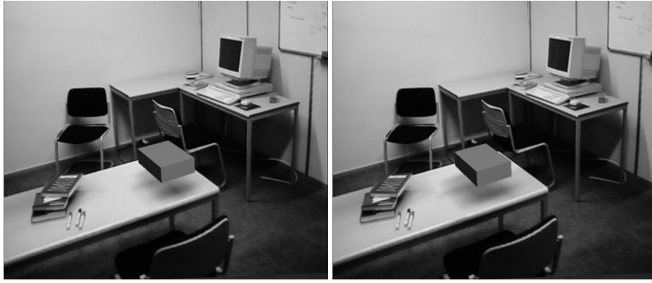
Fig. 4. (a) The complete CAR rendering using RVI texture polygons for display, including the CG object. (b) The CG object moves to the left: update takes 2.5 seconds. (See Colour Section).
