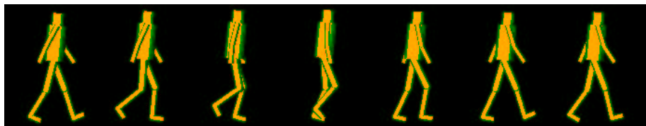
Figure 3: Snapshots of the motion, during a step. We define a step by the interval between two consecutive stands, the cycle is made of two steps.
