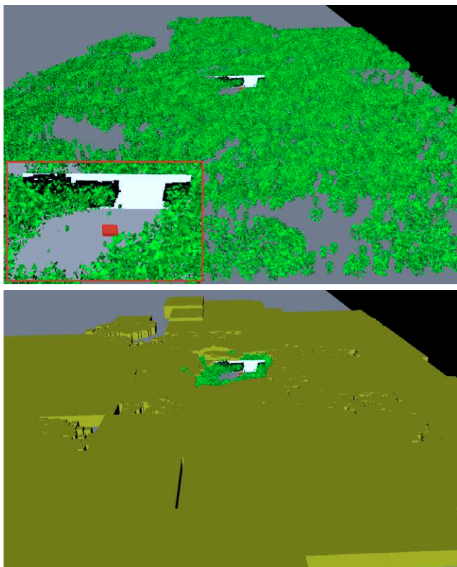
Figure 1: Top: A 7.8 M poly forest scene (only a tenth of the leaves are rendered here). The inset shows a close-up on the viewing cell (in red) and one of the projection planes. Bottom: Visibility computation from the view cell. In yellow we show the nodes of the hierarchy of bounding boxes culled by our method. We also show one of the projection planes used.
