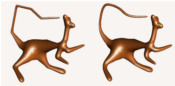
Figure 7. A stylized kangaroo modeled using subdivision curve primitives. Two different levels of detail are shown.
