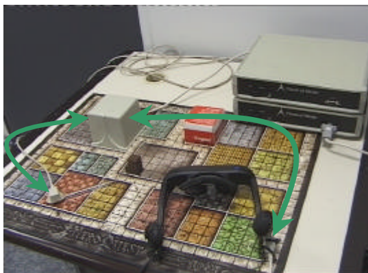
Fig5. Hardware use for the developed prototype. We can notice a HMD I-glasses, a pen, and the Flock of Birds systems ( an emitter, 2 receptors, and control unit).
