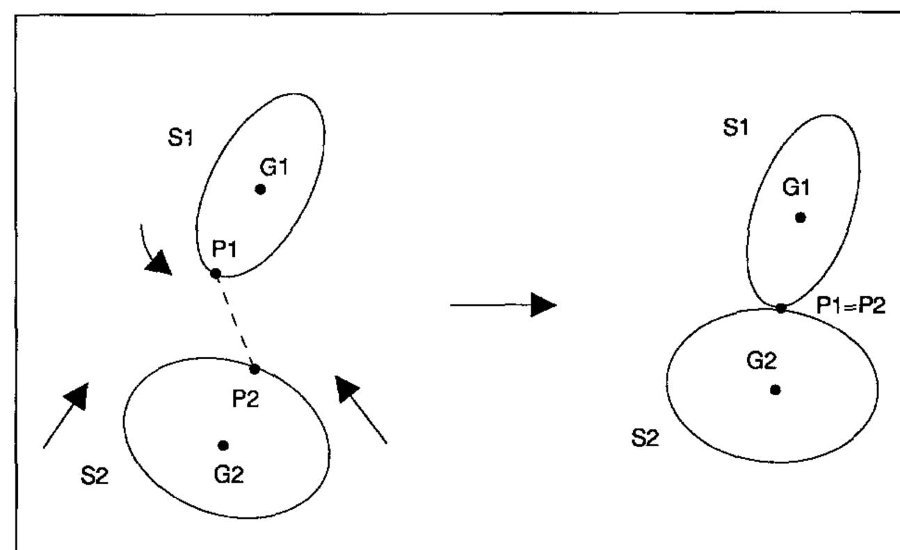
Fig. 1. A "point to point" constraint between two solids
