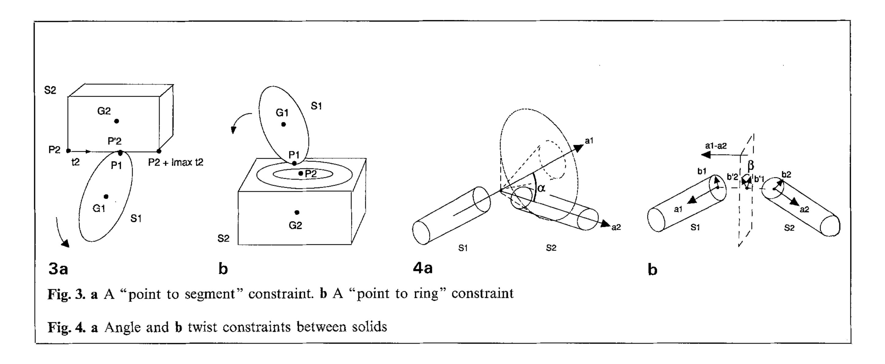
The displacements of  $S_1$  and  $S_2$  associated with this constraint at each iteration of the constraint processing are computed by replacing  $P_2$  in the equations that give the small rotation and the small translation with the point  $P_2'$  of the segment  $[P_2 + \lambda_{\min} \vec{t_2}, P_2 + \lambda_{\max} \vec{t_2}]$  that is the closest to  $P_1$ . Thus,  $S_1$  will be free to translate along the permissible segment of  $S_2$  (Fig. 3a).
