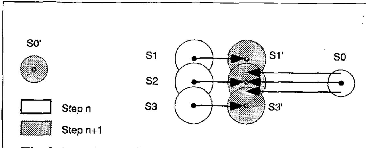
Fig. 2. For these solids, summing the translations associated with each constraint would move them farther away from a solution at each iteration
