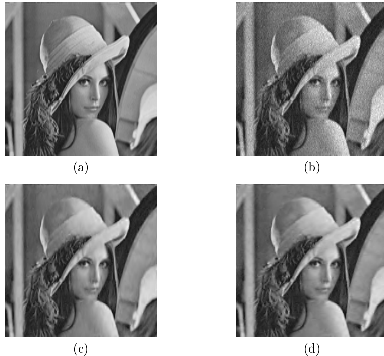
Figure 18: Results of the anisotropic wavelet transform. (a) is the original image with a sampling factor \alpha = 2 , (b) is the blur and noisy observation, (c) is the result obtained with an isotropic wavelet prior (actually the dual-tree complex wavelet prior that we have proposed in this paper) ( PSNR = 30.7 dB) and (d) is the result obtained with an anisotropic version of this wavelet transform ( PSNR = 30.2 dB).
