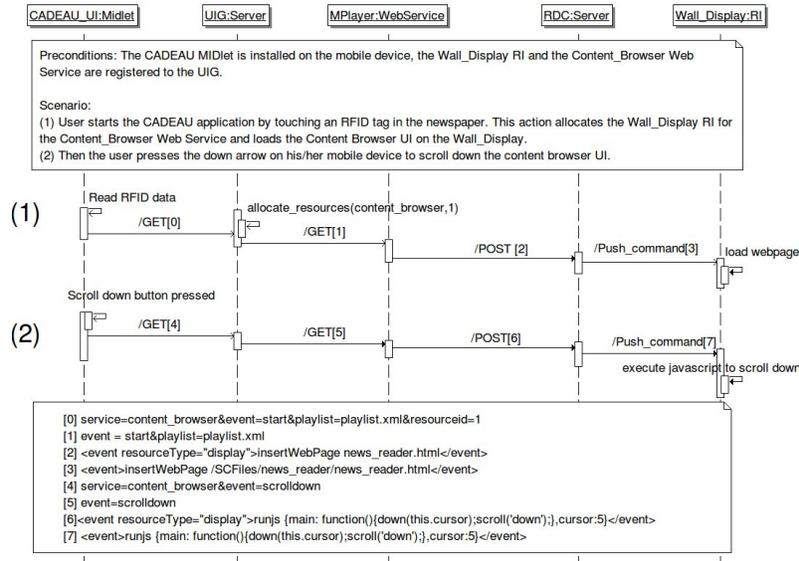
Fig. 11: Communication between the subsystems of CADEAU.
