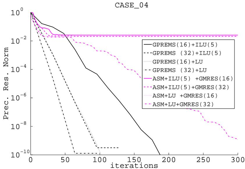
Figure 13: The multiplicative Schwarz approach (GPREMS) compared to the restricted additive Schwarz (ASM) on CASE\_004; 16 and 32 vectors in the Krylov subspace at each restart; 4 subdomains (block diagonal partitioning in GPREMS and Parmetis for ASM); local systems solved with different accuracies ( $ILU(5)$  and LU)
