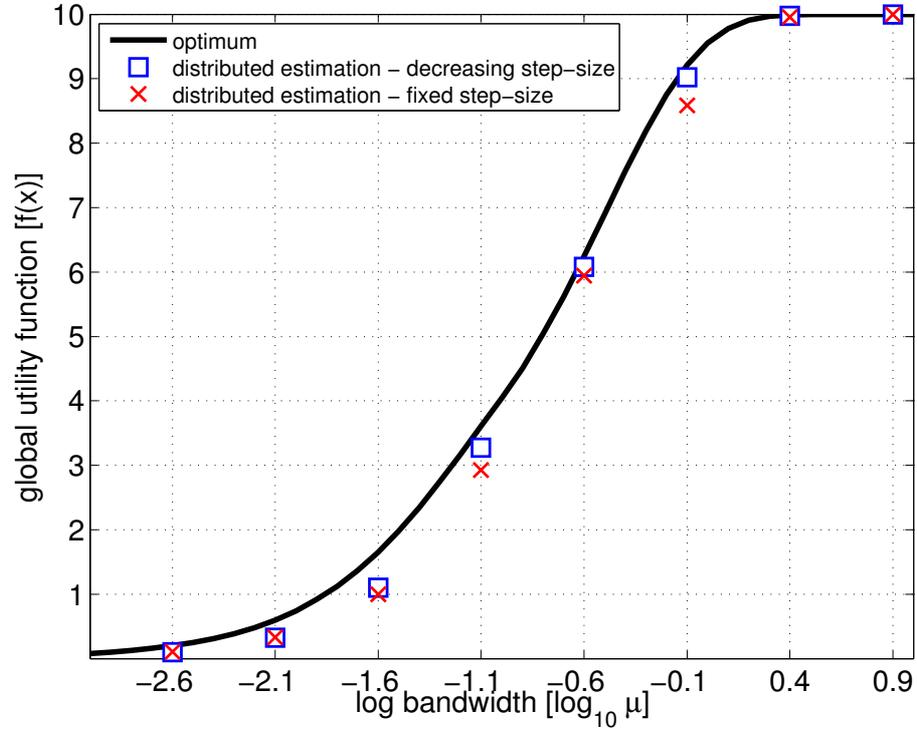
Figure 6: Theoretical maximum of the utility function *vs* utility of the rate allocation obtained with the distributed sub-gradient method for eight different bandwidth's values.
