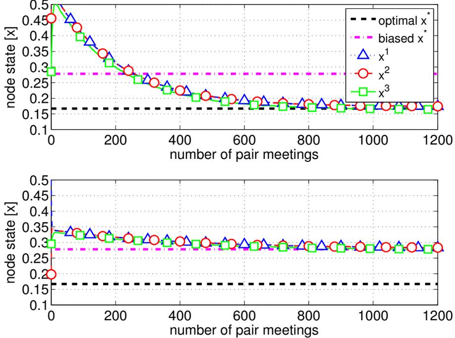
Figure 2: Toy example, convergence of the three estimates in case of fixed step-size  $\gamma = 25 \cdot 10^{-4}$ . Results have been averaged over 100 simulation runs. Top graph: synchronous updates. Bottom graph: asynchronous updates.
