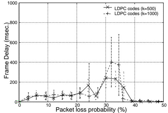
Fig. 5. Frame delay with LDPC codes ( $k = 500, 1000$ )
