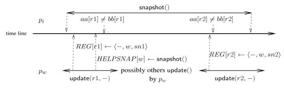
Figure 1: A snapshot with two concurrent updates by the same process
