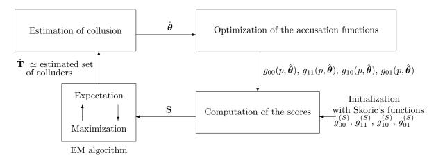
Figure 1. Computation of new accusation sum functions
