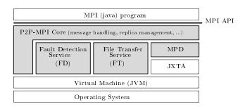
Figure 1. P2P-MPI structure.
