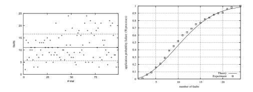
Figure 5. Number of faults leading to a crash for 100 experiments (p = 50, r = 2) (left), Comparison of experimental numbers of faults with theoretical count (right)
