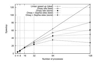
Figure 9. Ray-tracer speedups when run on a single site and on two distant sites.
