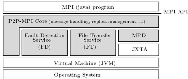
Figure 1. P2P-MPI structure.
