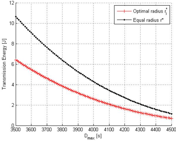
Fig. 2. Optimal radii  $r_i^*$  versus the number of messages  $M_i$  for each sensor  $i$  (top); transmission energy versus the maximum delay  $D_{max}$  both for optimal radii  $r_i^*$  and equal radii  $r^*$  (bottom).
