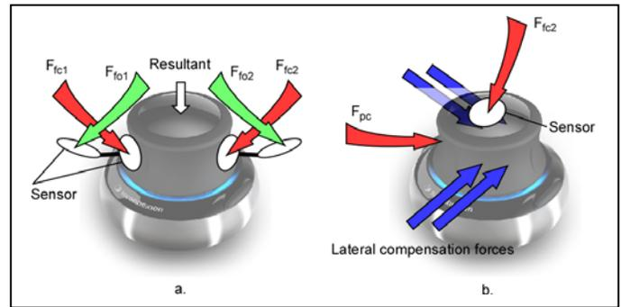
Figure 6: Force compensation (here with two fingers). In red: closing pressure ( $F_{fc}$  for the fingers and  $F_{pc}$  for the palm), in green: opening pressure ( $F_{fo}$  for the fingers), in blue: compensation forces. a: opposite distribution of forces when opening/closing simultaneously two fingers; no compensation needed. b: if the sensor is on the top of the device, it is necessary to apply strong lateral forces to compensate  $F_{fc2}$  and maintain the desired wrist configuration.
