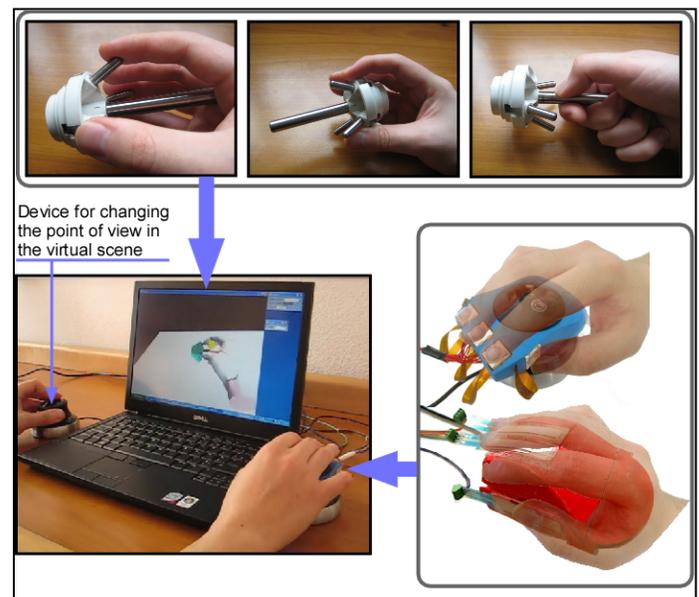
**Figure 1: Example of manipulation tasks that can be achieved with the HandNavigator, an immersive peripheral device for grasping virtual objects. Several prototypes using different sensors' technologies are presented.**
