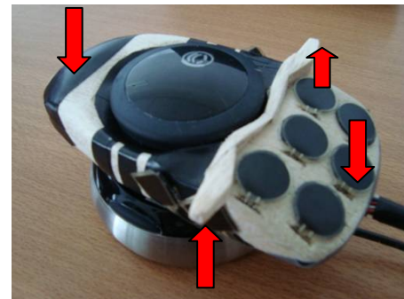
(b) Computer mouse shape. The arrows show where the user can apply forces to help force compensation.
