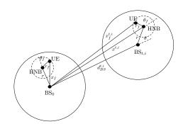
Fig. 3. Geometry of femto-UEs to the target macrocell  $BS_0$ .
