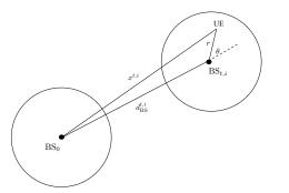
Fig. 2. Geometry of a neighboring-cell UE to the target macrocell  $BS_0$ .
