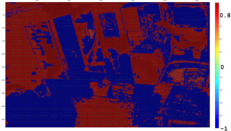
Figure 5. Pseudo color plot of lower bound on intensity reduction ratio of red channel of the scene in figure 4. Blue means the region does not have learning Data. Dark red means the region have a high lower bound, yellow means the region have a low lower bound
