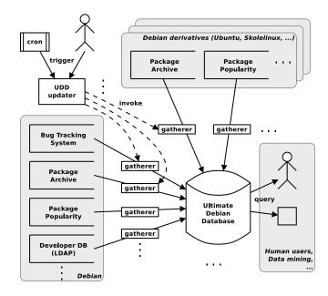
Figure 1. Data flow in the Ultimate Debian Database
