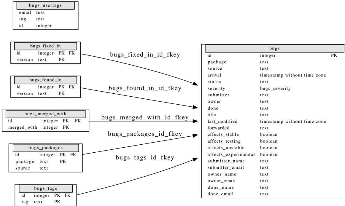
Figure 3. UDD schema corresponding to the Debian bug tracking system. All the information stored in the original service are available from UDD, as well as some convenience columns (source, affects\_unstable, affects\_testing, etc.) which are computed during data injection.
