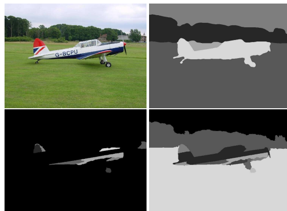
Figure 4. Example of optimal parameters extraction. From left to right and from top to bottom: input image, manual segmentation, segmentation with default parameters, segmentation after optimal parameters extraction.
