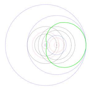
Figure 5: Two toleranced balls and their bisector which is a degree four algebraic curve—green curve. Dashed circles corresponding to the inner and outer balls. Dotted circles correspond to the solutions of a degree four equation: blue ones are toleranced tangent circles, red ones are algebraic artifacts.
