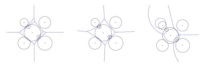
Figure 1: Curved Voronoi diagrams of 7 circles / weighted points. (Left) Power diagram  $d(S_i(c_i, r_i), p) = ||p - c_i||^2 - r_i^2$ . (Middle) Apollonius diagram :  $d(S_i(c_i, r_i), p) = ||p - c_i|| - r_i$  (Right) Möbius diagram :  $d(S_i(c_i, a_i, r_i), p) = a_i ||p - c_i||^2 - r_i^2$ .
