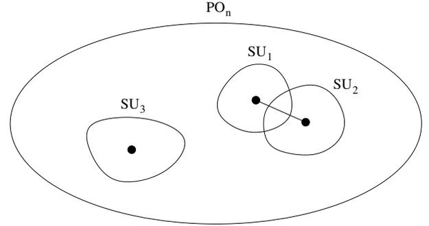
Fig. 1. Example CRN scenario with one primary operator ( $PO_n$ ) and 3 secondary users ( $SU_1, SU_2$  and  $SU_3$ ).  $SU_1$  and  $SU_2$  interfere with each other on channel  $n$ , while  $SU_3$  does not interfere with any other user.
