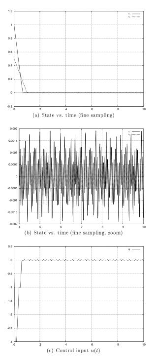
Figure 3: Simulation of the system (10) with  $\varphi(t) = \phi \sin \omega t$ ,  $\phi = 0.1$ ,  $\omega = 100$ .
