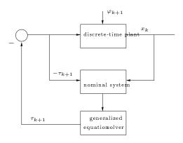
Figure 1: The discrete-time closed-loop system.
