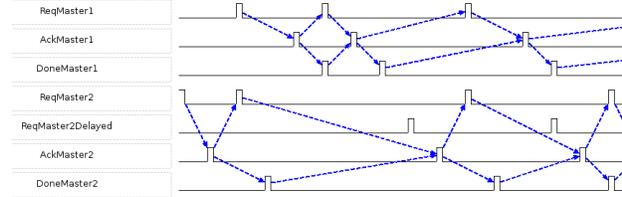
**Figure 4. Simulation of static priority system**
