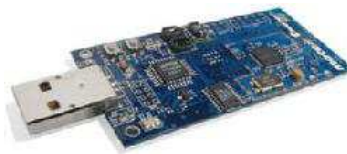
Figure 7: Tmote SKY platform from Crossbow
