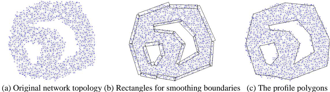
Figure 1: Profile polygons for a large-scale network.
