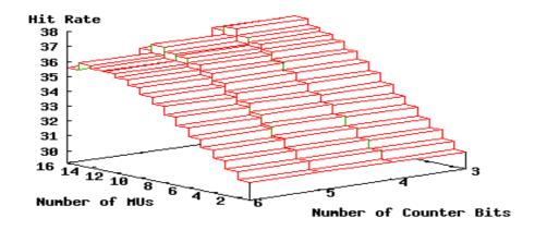
Figure 1: Hit rate of different LRU + Protected MU configurations
